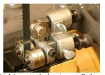
Full roller guides upper (left) and lower (right) are standard equipment. Both feature easy-to-adjust dials for making precise, tool-free adjustments of the side and thrust bearings.
